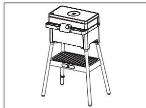
7| Place the appliance on the supporting legs. When rotating the wind and splash guard (1) and the oven door (4), secure them to ensure that they don't open.
